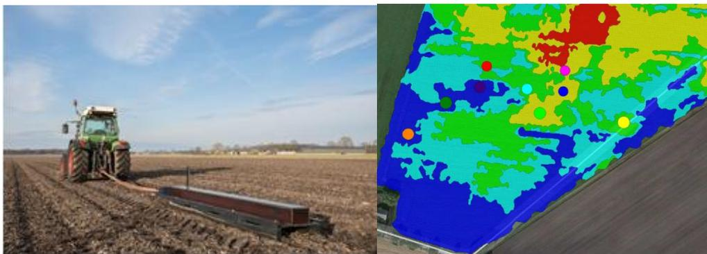
**Figure 4** On the left, a tractor scanning the soil with the DualEM sensor. On the right, soil scan result of the pilot field in Netherlands in 2016.
